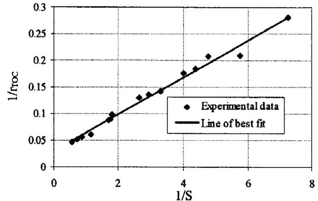
Figure 4. Monod kinetics parameter determination.
