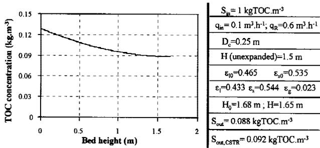
Figure 8. Example of calculation and concentration profile.
