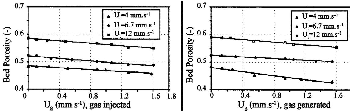
Figure 5. Influence of gas velocity on bed porosity at various liquid velocities for the two modes of gas introduction.
