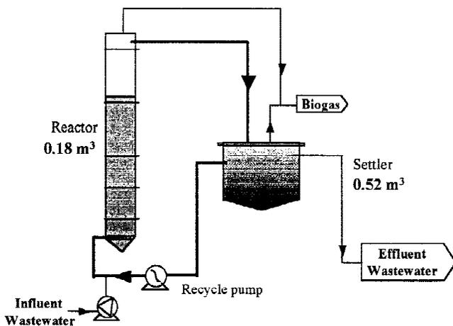
Figure 2. Anaerobic fluidized-bed reactor treating wine distillery wastewater.
