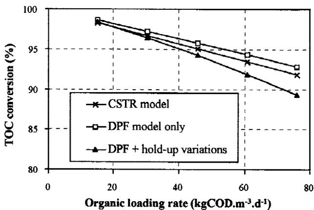
Figure 9. Influence of organic loading rate on reactor performance. Reactor diameter: 2 m; initial bed height: 10 m; inlet concentration  $1 \text{ kgTOC m}^{-3}$  ( $2.5 \text{ kgCOD m}^{-3}$ ).
