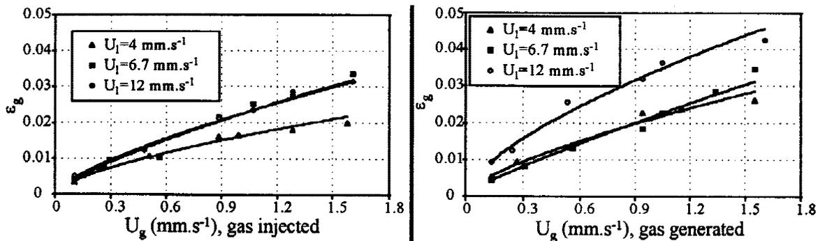
Figure 6. Influence of gas velocity on gas hold-up for the two modes of gas introduction.
