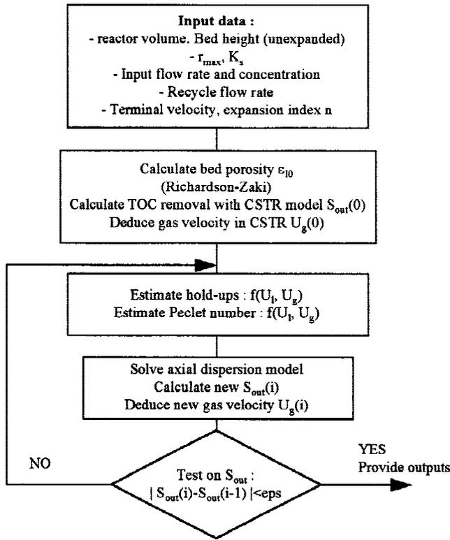
Figure 3. Iterative procedure for gas-producing fluidized-bed performance calculation.
