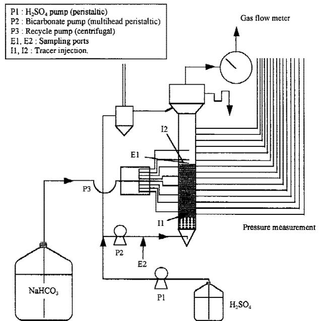
Figure 1. Experimental device for the hydrodynamic studies.
