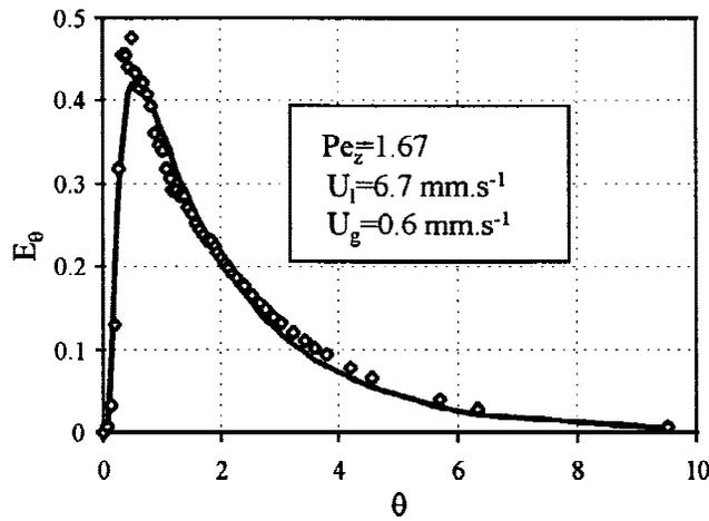
**Figure 7.** Example of experimental pulse response and corresponding axial dispersion model.
