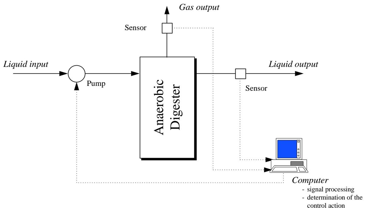
**Figure 1** : Loop for the control of processes.
