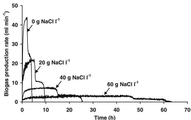
**Fig. 2** Evolution of biogas production rate during standard cycles (reaction step) with increasing NaCl concentrations. Reactor operating with ethanol
