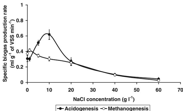
**Fig. 3** Evolution of specific biogas production rate due to acidogenesis and methanogenesis with increasing NaCl concentrations using ethanol as a substrate
