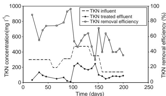
Fig. 7. Evolution of TKN concentration in the influent and treated effluent and evolution of TKN removal yield during the experiment.
