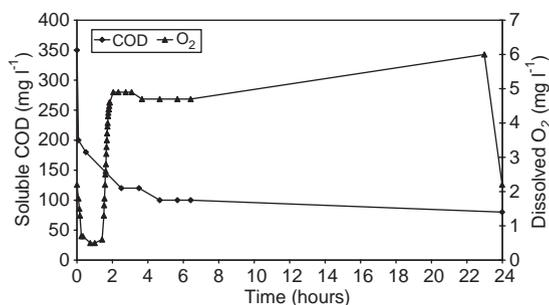
Fig. 6. Evolution of soluble COD and dissolved  $\text{O}_2$  during one cycle of operation of the SBR.
