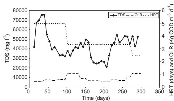
Fig. 3. Evolution of HRT, OLR and TDS concentration in the reactor during the experiment.
