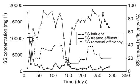
Fig. 8. Evolution of SS concentration in the influent and treated effluent and evolution of SS removal yield during the experiment.
