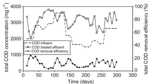
Fig. 4. Evolution of total COD concentration in the influent and treated effluent and evolution of COD removal yield during the experiment.
