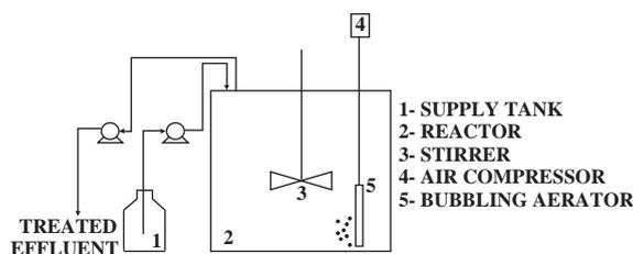
Fig. 2. Lab-scale aerobic SBR.
