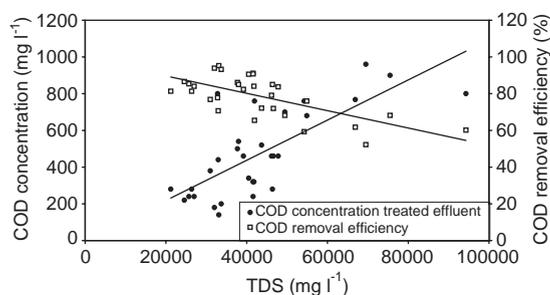
Fig. 5. Evolution of COD concentration in the treated effluent and COD removal yield with TDS concentration.
