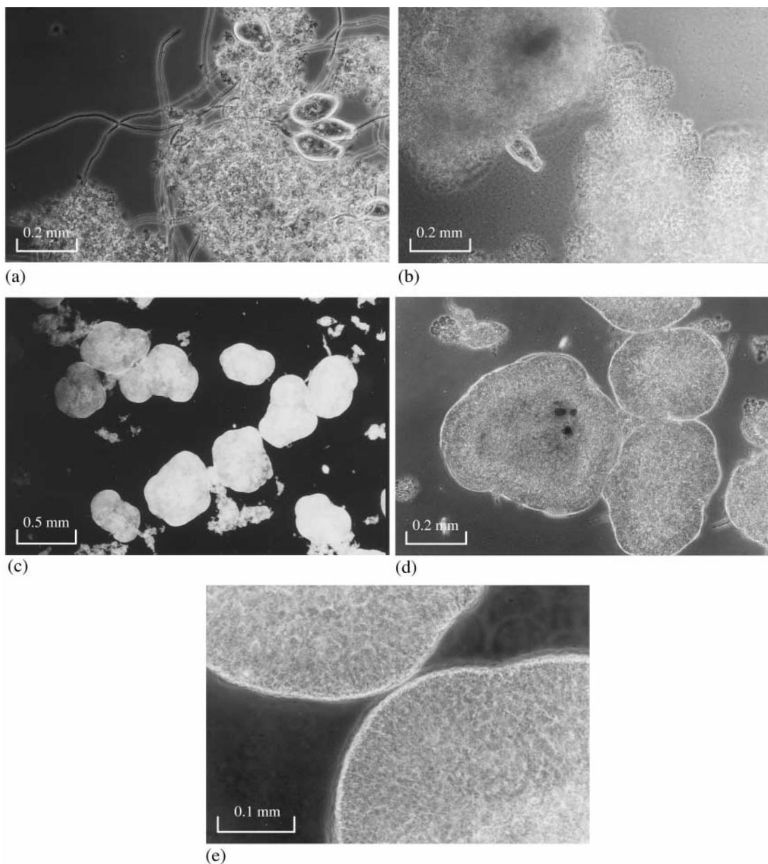
Fig. 1. Evolution of the activated sludge in the reactor: (a) seeding sludge; (b) floc-like sludge; (c), (d), (e) granular sludge.
