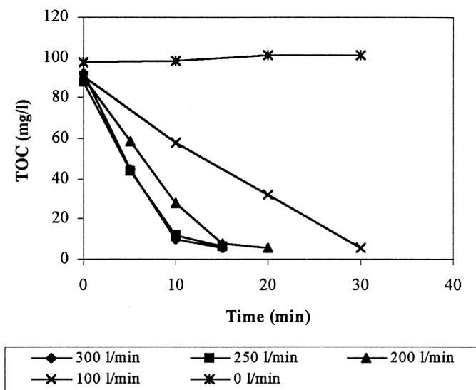
Fig. 2. Kinetic study of granular sludge under different aeration conditions.
